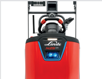
Linde BlueSpot™ and front LED light
