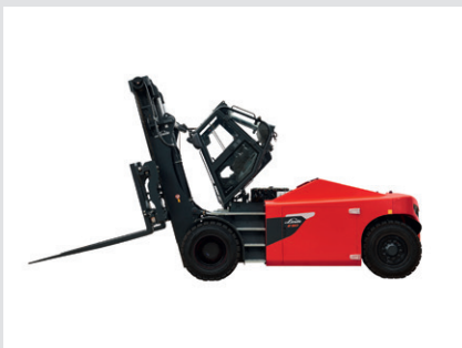
Service access through tiltable cabin
